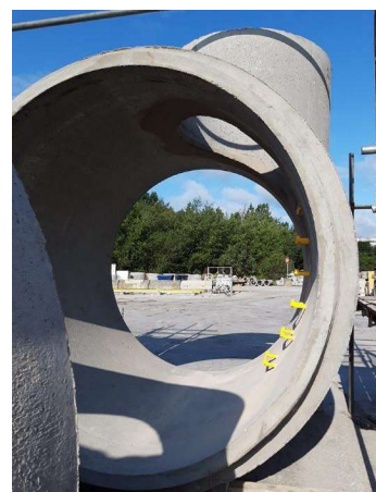
Figure 2. Side entry unit used as part of a concrete attenuation tank.
